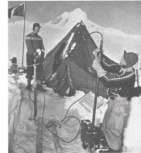
Electro-thermic glacier drilling on the Juneau Icefield.
