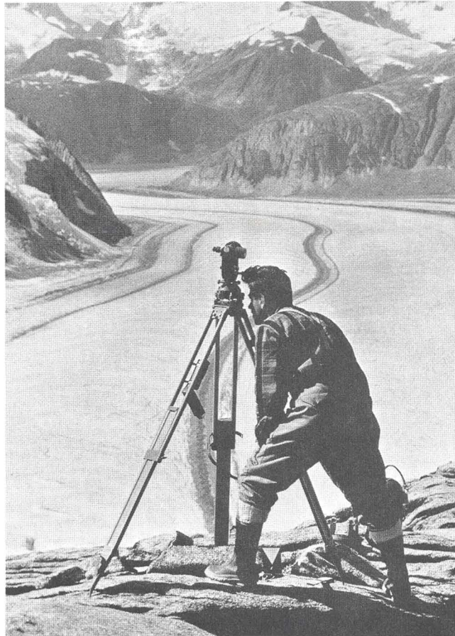
Theodolite station in Gilkey Canyon for the National Geographic Society's regional glacier survey.
