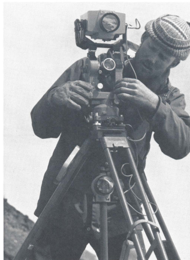
Student using T-2 and EDM Survey instruments in Camp 17 sector.
