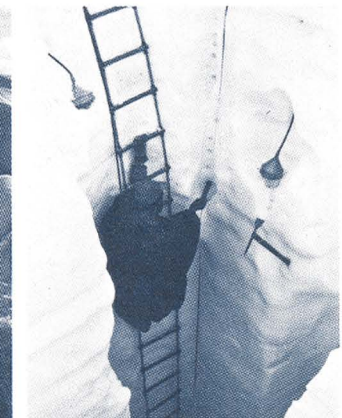
Measuring snow & firn stratigraphy at test pit site.
