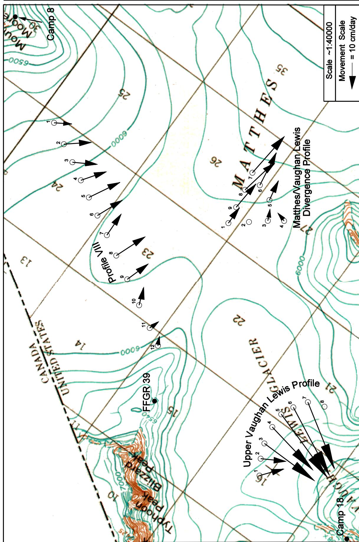
Figure C3: Movement profiles on the high plateau
