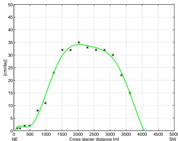
Fig. 7: Profile VII - measured (\*) and adjusted (-) velocities
