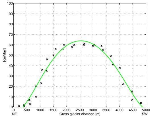
Fig. 3: Profile IV - measured (\*) and adjusted (-) velocities
