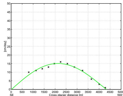
Fig. 9: Profile VIII - measured (\*) and adjusted (-) velocity
