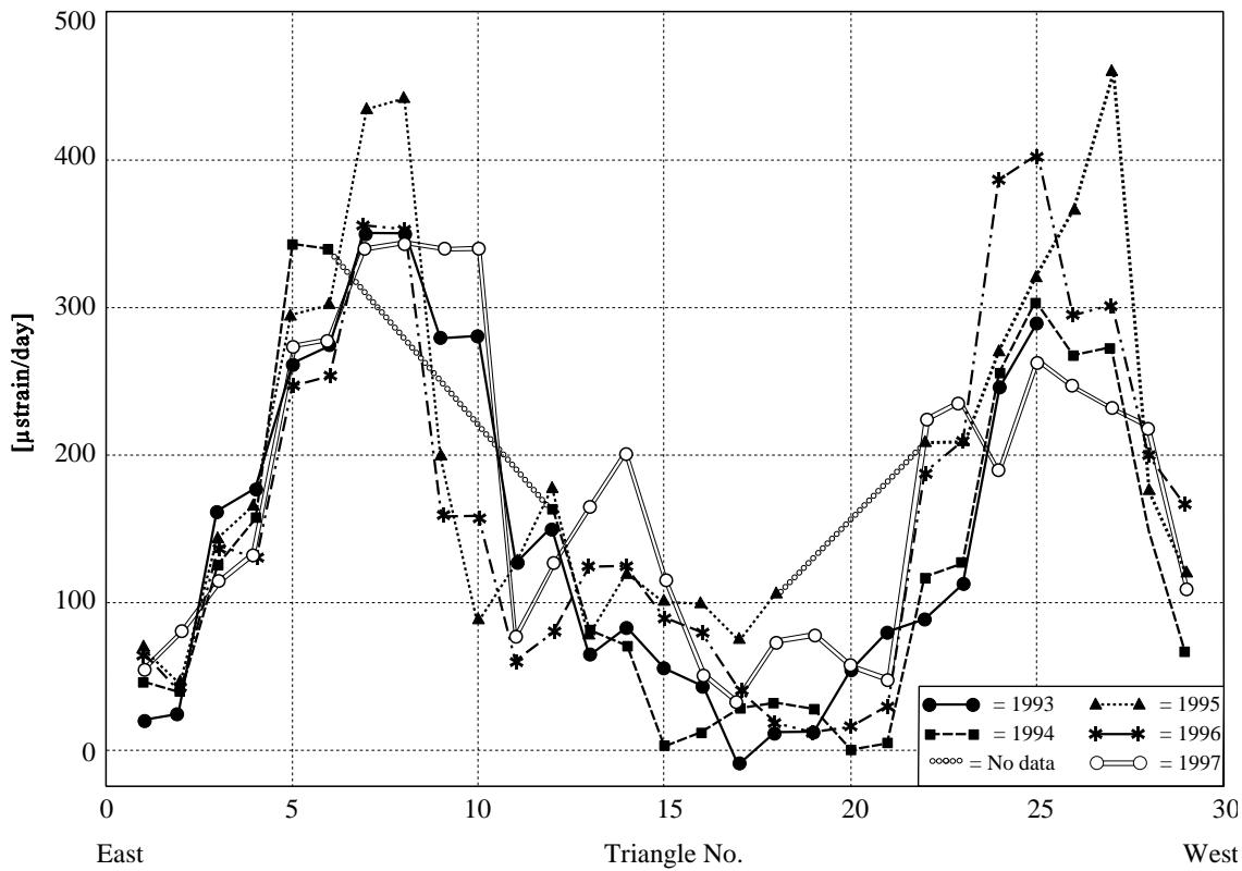
Fig. 18: Maximum principle strain rate ( $e_1$ ) on Profile IV, 1993-1997.
