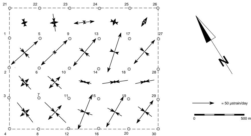
Fig. 19: Strain ellipses for the Divide Grid Profile
