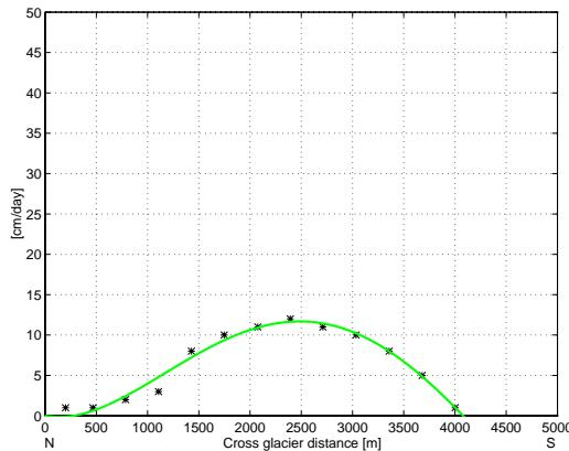
Fig. 5a: Profile VIc - measured (\*) and adjusted (-) velocities
