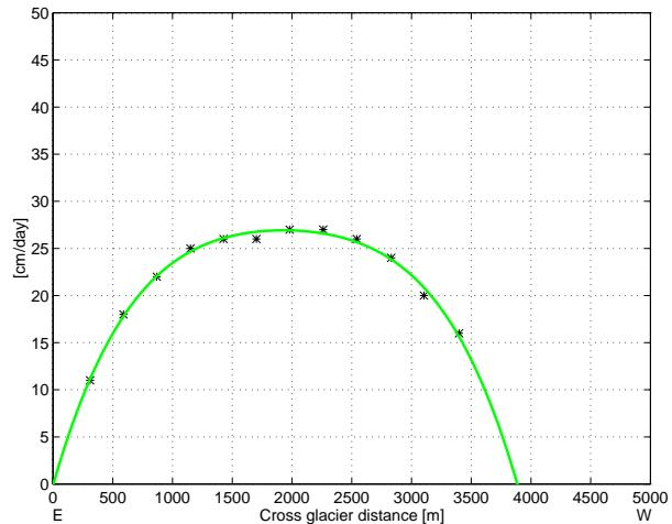
Fig. 11: Profile XI - measured (\*) and adjusted (-) velocity
