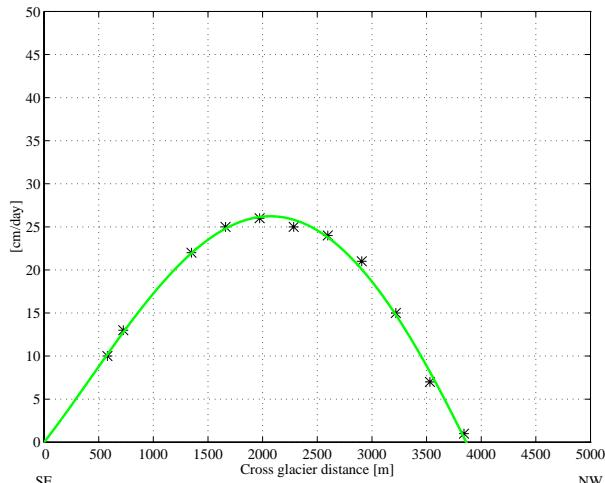
Fig. 2: Profile III - measured (\*) and adjusted (-) velocities
