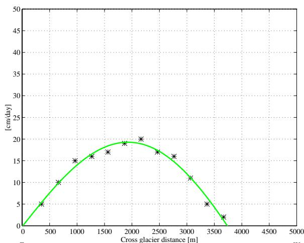
Fig. 3: Profile IIIa - measured (\*) and adjusted (-) velocities
