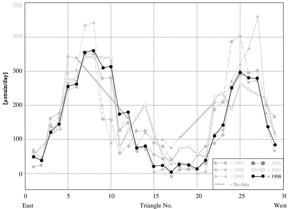
Fig. 18: Maximum principle strain rate ( $e_1$ ) at Profile IV, 1993-1998. Data for 1998 are in black
