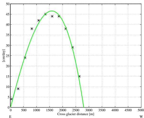
Fig. 10: Profile VIIb - measured (\*) and adjusted (-) velocities
