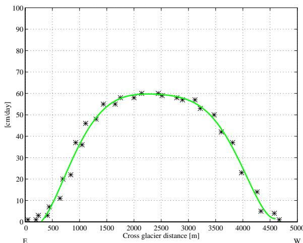
Fig. 4: Profile IV - measured (\*) and adjusted (-) velocities
