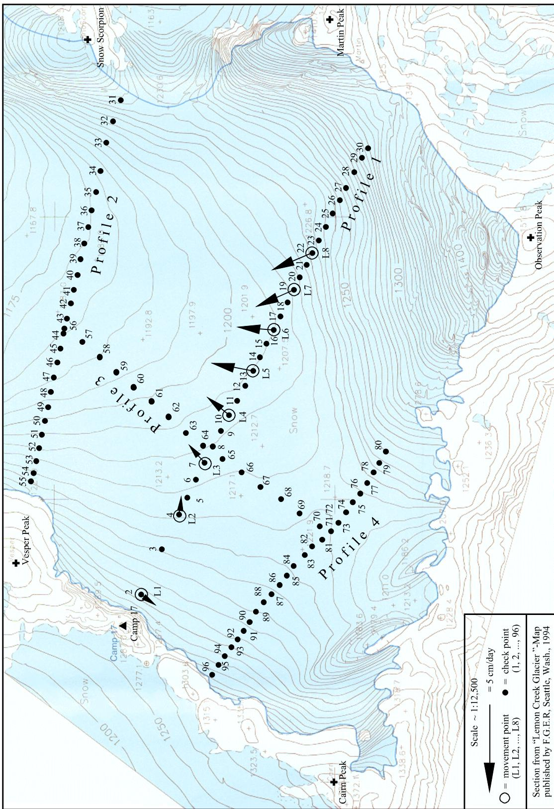
Fig. 24: Movement vectors and locations of height comparison profiles on the Lemon Creek Glacier
