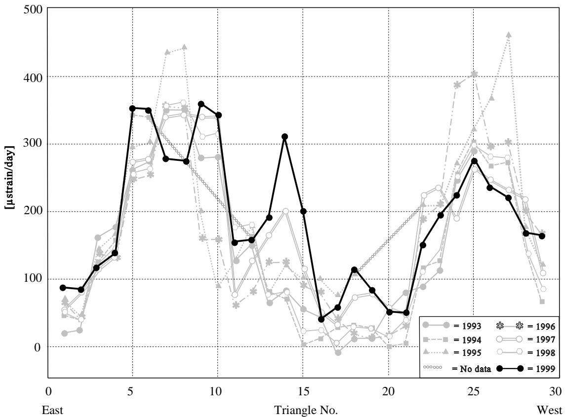
Fig. 25: Maximum principle strain rate ( $e_1$ ) at Profile IV, 1993-1999. Data for 1999 are in black
