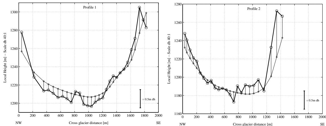
Fig. 23, part I: Lemon Creek Glacier height change 1998-1999: Profiles 1, 2. Thin line: glacier surface 1998, bold line: glacier surface 1999.
