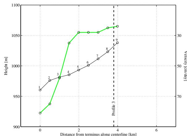
Fig. 11: Longitudinal Profile Demorest Glacier, southern part. Measured velocities (grey) and heights (black).
