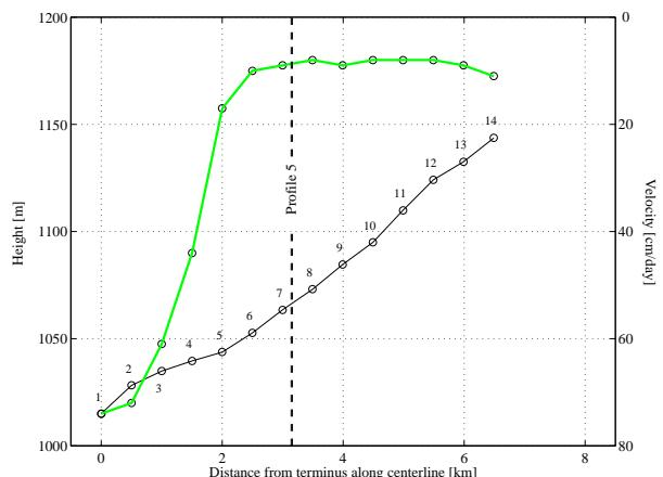
Fig. 15: Longitudinal Profile Taku Glacier SW-Branch.
