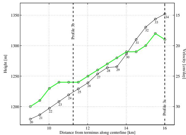
Fig. 10: Longitudinal Profile Demorest Glacier, northern part. Measured velocities (grey) and heights (black).
