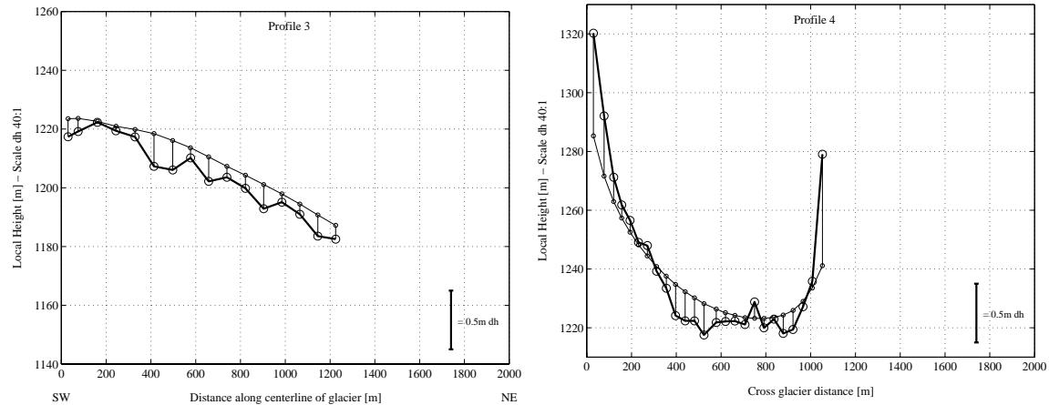
Fig. 23, part II: Lemon Creek Glacier height change 1998-1999: Profiles 3, 4. Thin line: glacier surface 1998, bold line: glacier surface 1999.
