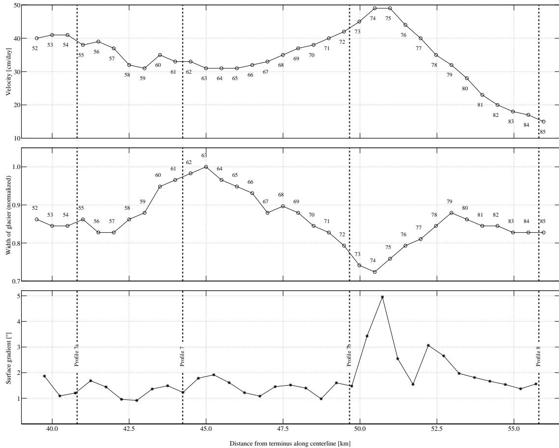
Fig. 13: Longitudinal Profile Matthes Glacier. Measured velocities, glacier width and surface gradients
