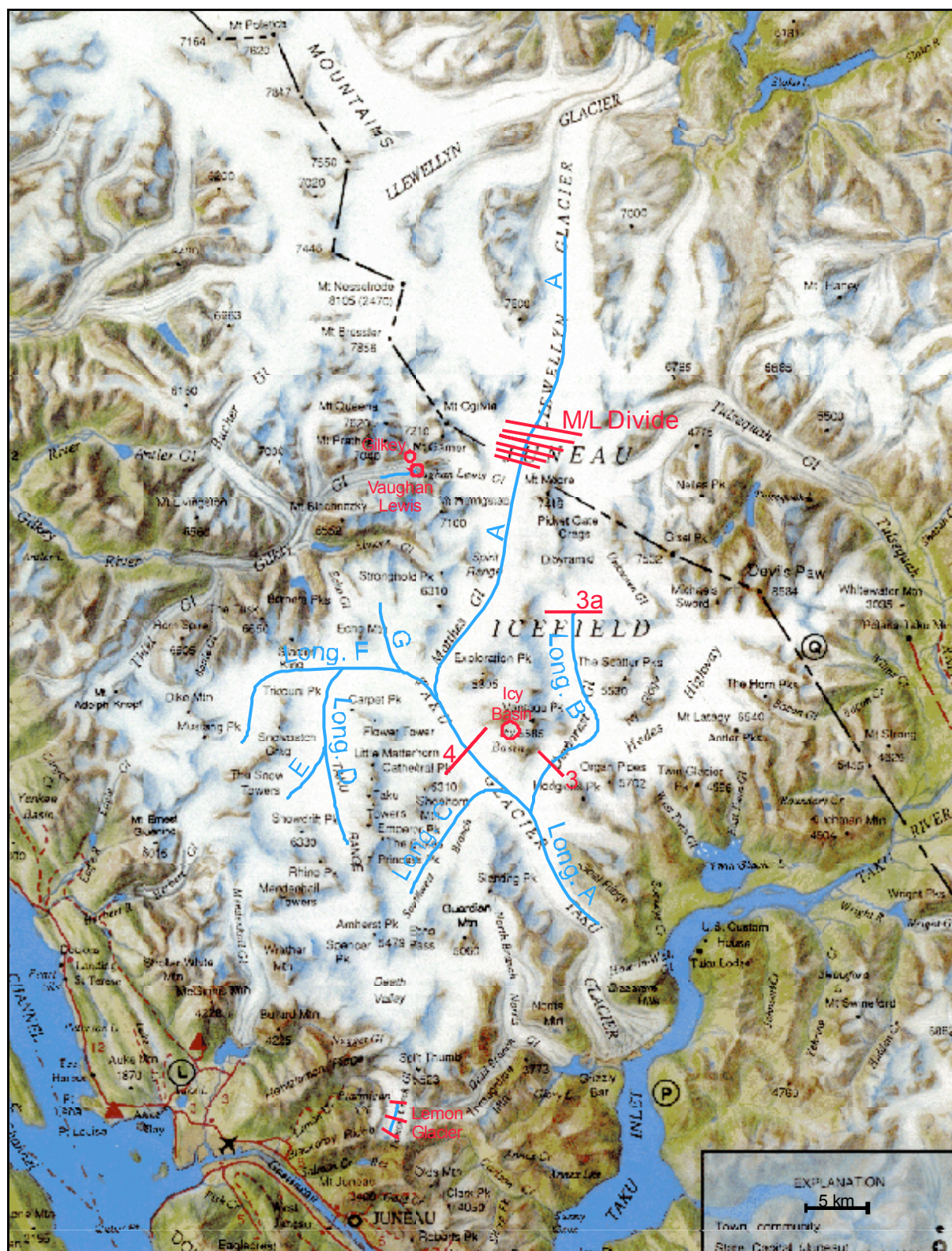
Figure 2: Location of transverse and longitudinal profiles surveyed during the 2001 JIRP field season.
