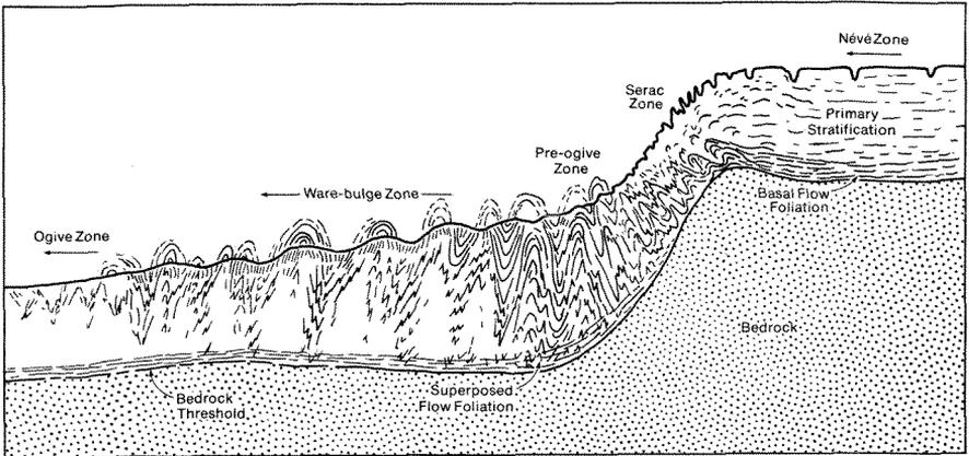
FIG. 16. Schematic long-section, showing evolution of folded tectonic foliation on Vaughan Lewis Glacier and relationship to changing dip of folia in wave-bulge and ogive zones.
