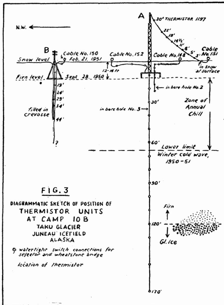
crevasse and marked with a wooden tower for future reference. At Camp 8 B another string of thermistors was placed in a bore-hole. The unit spacing on these was the same as noted for No. 148, thus permitting measurement of the temperature gradient in the highest névé at increments of 1 to 5 feet (position below surface shown in Fig. 9).
