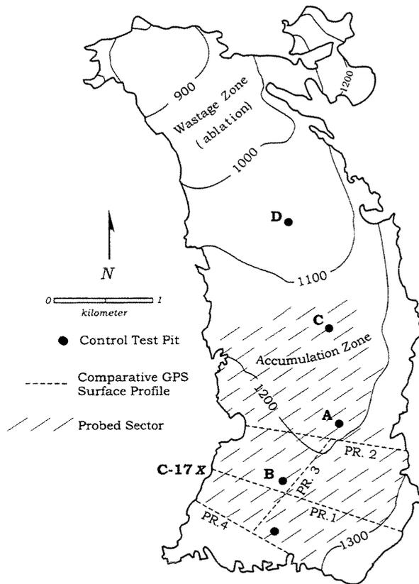
Fig. 5. Location of standard test-pit sites and comparative leveling GPS profiles in main upper névé.
