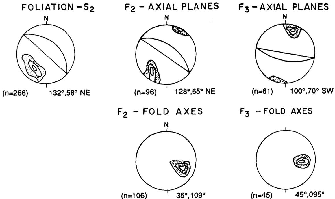
FIG. 4. Equal-area-net plots of  $F_2$  and  $F_3$  structures in the AJ mine (lower hemisphere projections). Contours indicate 1, 5, and 15 points per 1% area.
