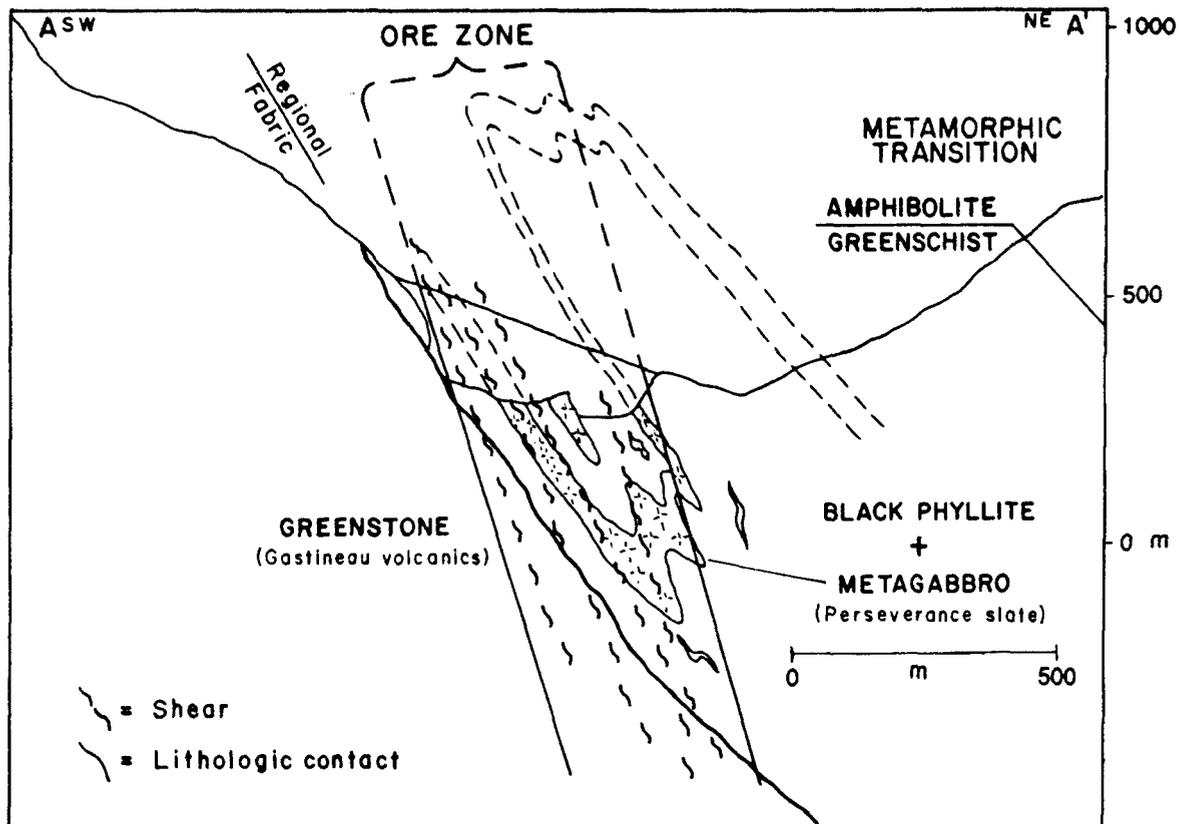
FIG. 3. Schematic cross section through the main ore zone in the AJ mine. Note the crosscutting geometry of the ore zones in relation to the regional fabric. Location of section A–A' shown in Fig. 2.
