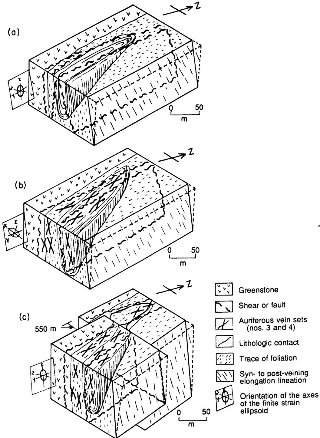
FIG. 11. Block diagrams showing the structural evolution of the AJ deposit. (a) Development of ductile shear zones. (b) Auriferous veining within the shear zone and in areas of infolded metagabbro and phyllite. (c) Postmineralization brittle deformation with left-lateral offset of the orebody along the Silverbow fault.
