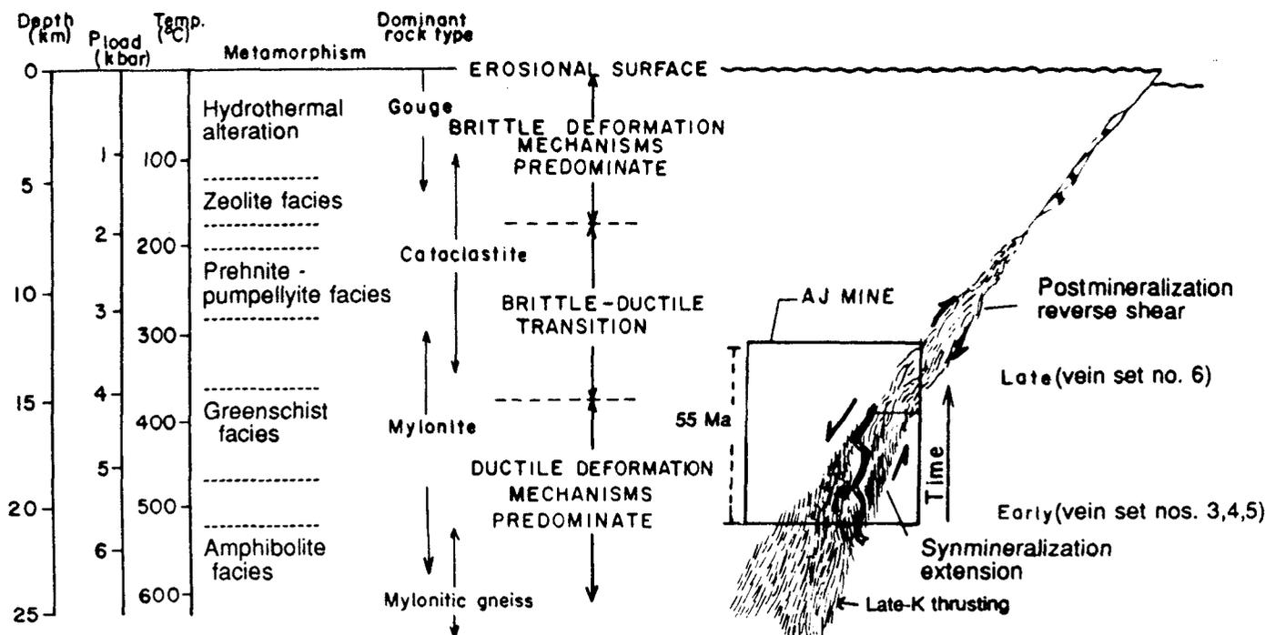
FIG. 10. Pressure and temperature regimes and the corresponding shear fractures controlling vein geometries. Note the inferred progression of veining at the AJ deposit (after Sibson 1977, 1983; Colvine *et al.* 1988).
