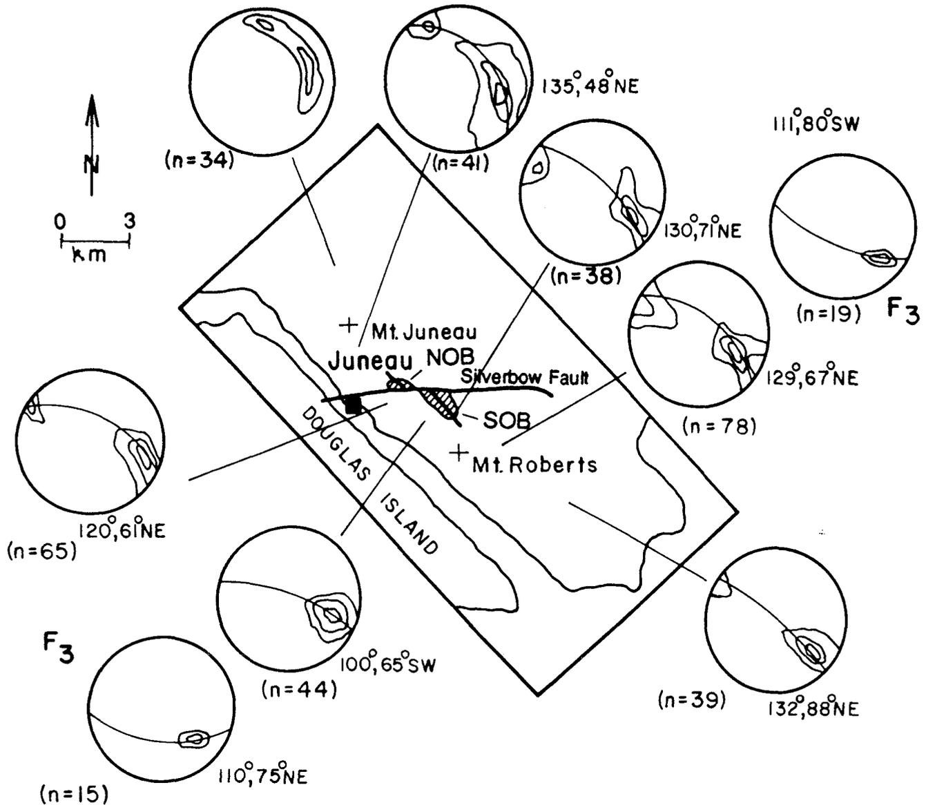
FIG. 5. Plan map with stereonets of fold axes in the AJ mine area, showing the change in fold axis plunge from northwest-southeast across the study area. All orientations are of  $F_2$  folds except as noted. NOB, North orebody; SOB, South orebody.
