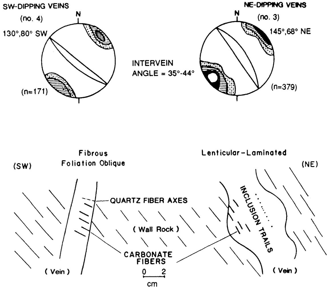
FIG. 7. Stereoplots of poles to planes and schematic sketch of sets 3 and 4 veins. Note the angular relations and the orientations of the mineral fibers. Contours indicate 1, 5, 15, and 25 points per 1% area.
