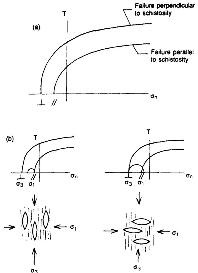
FIG. 9. (a) Mohr failure envelopes for failure normal to, and parallel with, schistosity. (b) Veining parallel to schistosity due to increased fluid pressure ( $p_f$ ) under maximum compressive stress perpendicular to the fabric. (c) Veining perpendicular to schistosity under the same stress configuration with greater fluid pressure (from Kerrich 1986).
