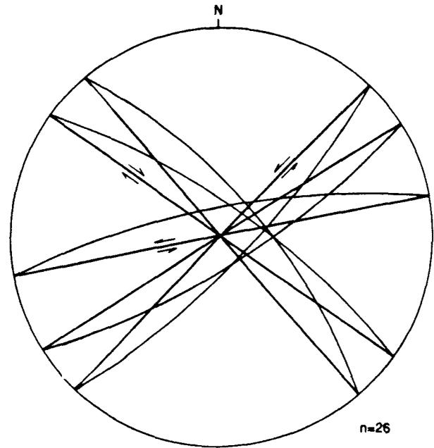
FIG. 6. Stereoplot of the principal shear orientations in the AJ mine (lower hemisphere projection).
