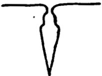
e. Snow bridge is broken by melting and further opening
