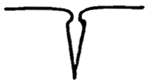
c. Snow bridge is broken in center by melting and by further opening of crevasse
